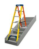
\*\*Only use the ladder on uneven ground, steps or stairs if the rear stile height can be adjusted so that the treads are level.
